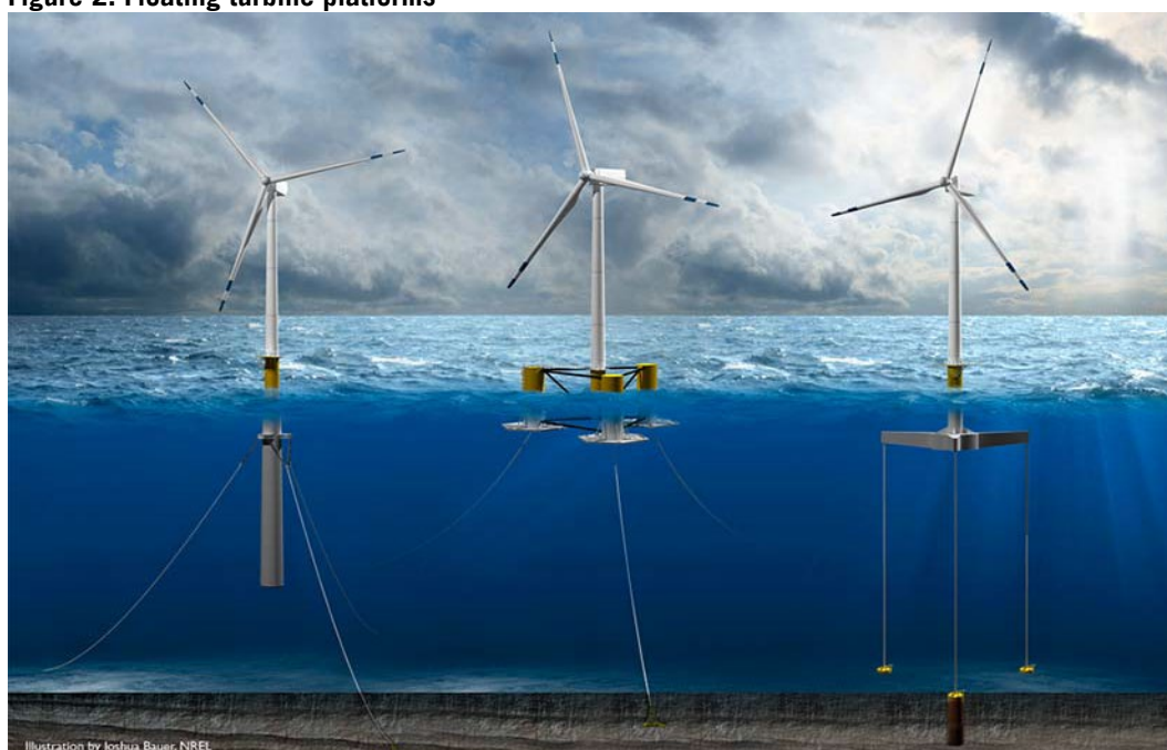
Figure 2: Floating turbine platforms 3
